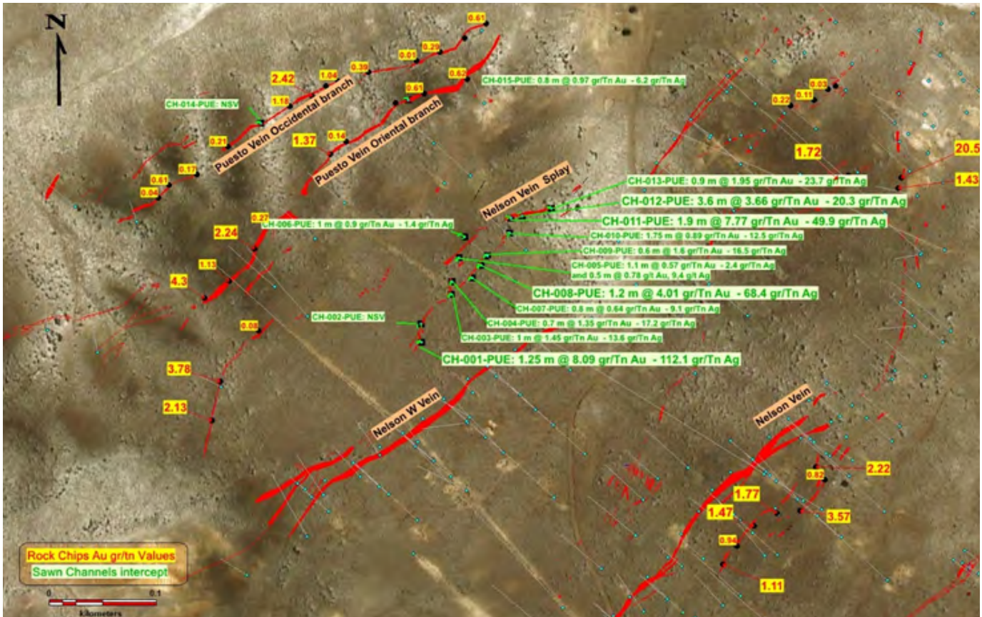
Fifteen channels and 49 chip sampling points
