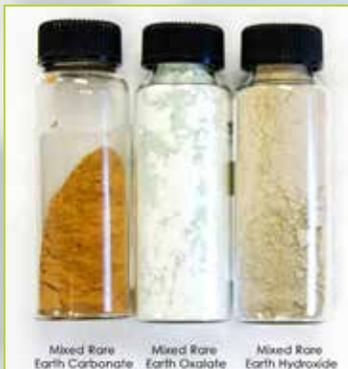
Montero announced in 2012 - its first **samples of concentrated Rare Earth chemical grade products produced from bastnaesite-rich carbonatite material from the Wigu Hill Rare Earth Project**. The products produced include a Mixed Rare Earth Carbonate, Oxalate and Hydroxide and importantly an individual Cerium Hydroxide product.
